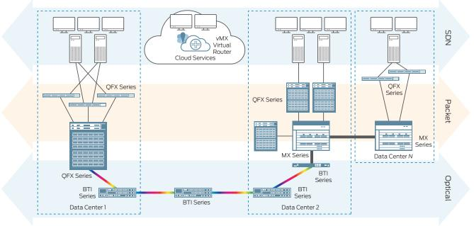
Figure 1: Open Cloud Interconnect components and layers
